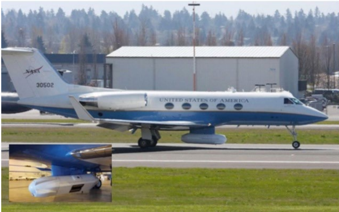
Figure 7.27. The NASA Gulfstream III with pod configured for Ka-band interferometry. Lower insert shows close-up with details of the IfSAR antennae.
