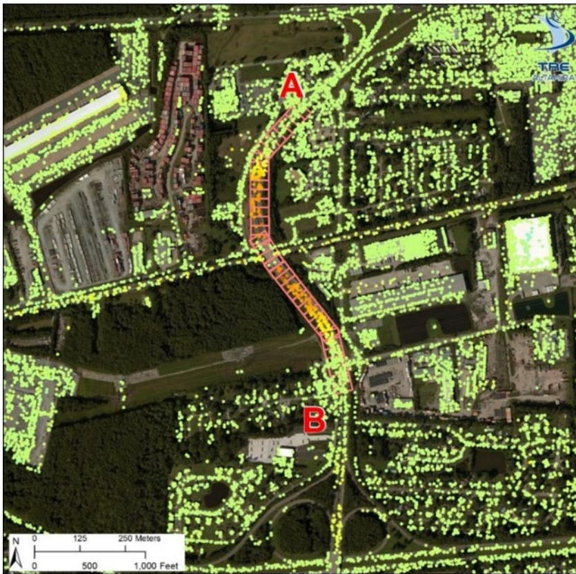
Figure 7.36. A cross-section over the George Washington overpass illustrating differential subsidence patterns in this area.
