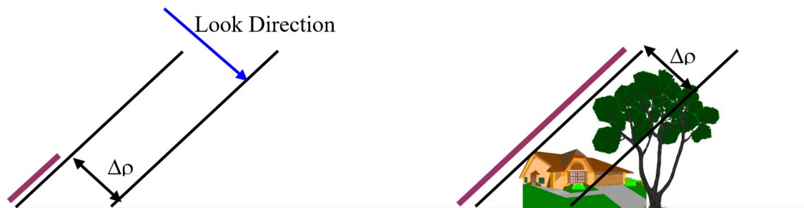
Figure 7.6. Vertical structure of scatterers within a resolution element due to vegetation or other structures present in the cell cause increased decorrelation. This form of decorrelation can be used to infer information about vertical structure within a resolution element. The increased decorrelation results from the increased size of the range cell projected back toward the direction of the radar (shown in magenta) when compared to a flat surface.
