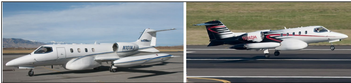
Figure 7.22. The STAR-3 (left image) and STAR-6 (right image) radars are flown on a Learjet 36 with the antennas mounted to an invar frame contained in the large dome on the underside of the aircraft. (Figures courtesy of Intermap Technologies Inc.)
